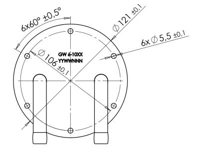
Accessories: Rubber sealing - WA 19677 Fixing screw stainless steel M5x16
